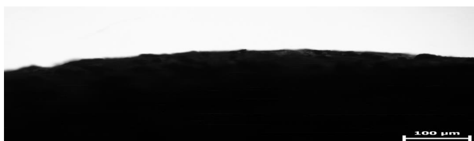
Fig. 3. Microstructure of surface irregularities h \approx 20 \pm 5 mkm C_8H_8 porous polystyrene foam + iron-manganese crust (IMC) - film of higher Mn oxides: pyrolusite MnO_2 , mangosite MnO , Mn_3O_4 , Mn(OH)_2 followed by its oxidation to manganate, MnO_x manganite ( 1 < x < 2 ), todorokite (Mn^{2+}, Ca)Mn^{4+}_3O_7 \cdot nH_2O after 10 functioning years.
