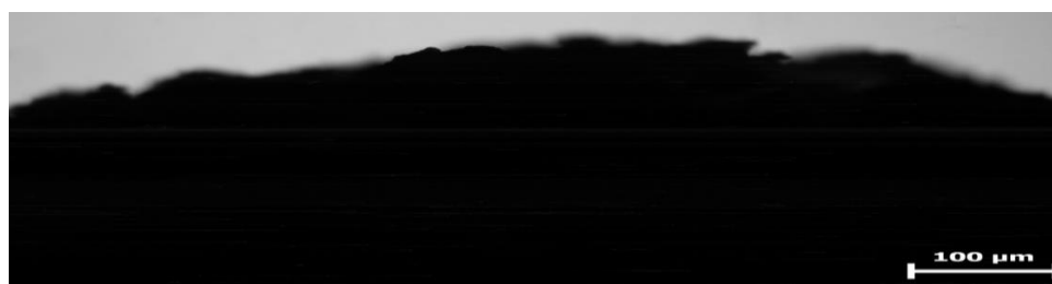
Fig. 2. Microstructure of surface irregularities h \approx 30 \pm 3 mkm C_8H_8 porous polystyrene foam + iron-manganese crust (IMC) - film of higher Mn oxides: pyrolusite MnO_2 , mangosite MnO , Mn_3O_4 , Mn(OH)_2 followed by its oxidation to manganate, MnO_x manganite ( 1 < x < 2 ), todorokite (Mn^{2+}, Ca)Mn^{4+}_3O_7 \cdot nH_2O after 10 functioning years.
