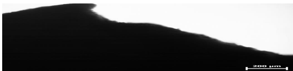
Fig. 4. Microstructure of surface irregularities h = 22 \pm 11 mkm of mineral zeolite Ca [Al_2Si_4O_{12}]x2H_2O before loading into the filter.
