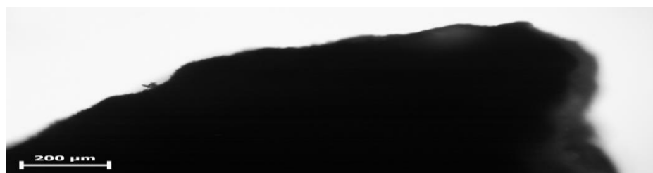
Fig. 5. Microstructure of surface irregularities h = 24 \pm 8 mkm of mineral zeolite Ca [Al_2Si_4O_{12}]x2H_2O before loading into the filter.
