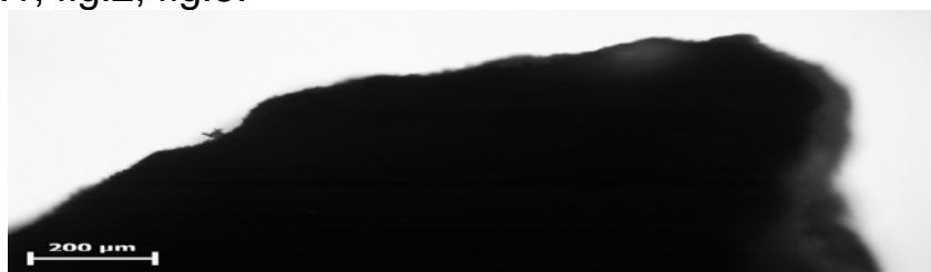
Fig. 1. Microstructure of surface irregularities h = 24 \pm 8 mkm of mineral zeolite \text{Ca}[\text{Al}_2\text{Si}_4\text{O}_{12}]\cdot 2\text{H}_2\text{O} before loading into the filter
