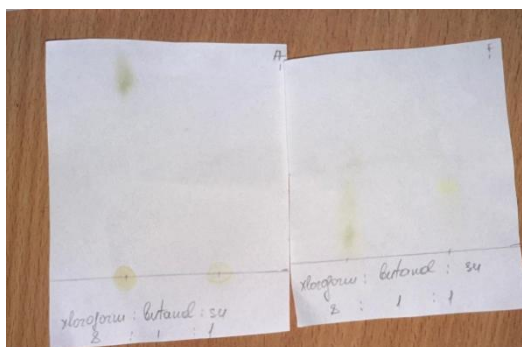
Figure 2. Chromatogram of leaf and root extracts obtained from Prangos acaulis and Prangos ferulacea , developed using a solvent system consisting of chloroform, butanol, and water in a ratio of 8:1:1
