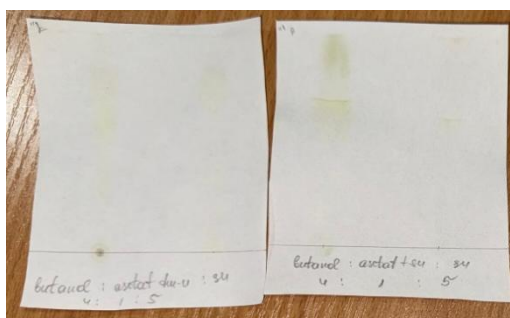
Figure 3. Chromatogram of leaf and root extracts obtained from Prangos acaulis and Prangos ferulacea , developed using a solvent system consisting of butanol, acetic acid, and water in a ratio of 4:1:5
